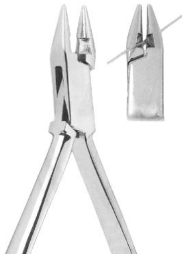
AS-7-5135 Bird beak pliers for bending round, square or rectangular wire up to 0,7 mm. (.028"). With cutter.
