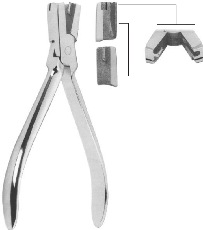
AS-7-5114 Nance Nance loop closing pliers, for bending of stop loops and special for Adams' clasps. Wires up to 0,7 mm. (.028").
